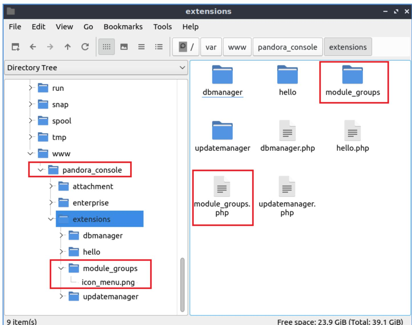
The instalation of extension is very easy, because the Pandora FMS search new extensions and add into system when new extension is found. You only copy all files of extensions into the directory extension in your [Pandora FMS Console instalation](#). But you must set the permissions for the Pandora FMS Console can read the files and subdirectories of extension.
