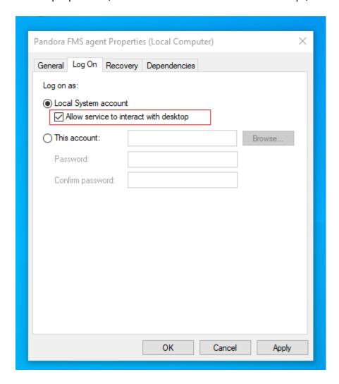
Pandora FMS, as a service, runs under the SYSTEM account and that the process executed will do so under that user and with that environment, so that if you need to run a specific process that needs to be used with a specific user, you must encapsulate in a script (.bat or similar) the previous processes to initialize the environment, environment variables, etc), and execute that script as action of the Watchdog.
