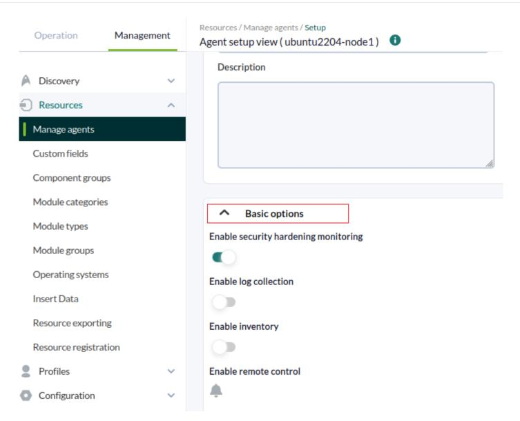
• Enable security hardening monitoring: It enables the plugin to strengthen security on the monitored device. The following options will be enabled in the configuration file:
