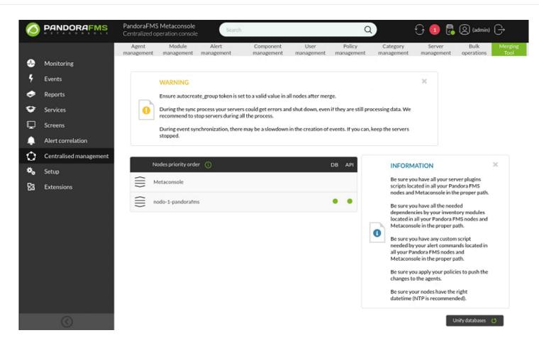
The Merging tool will merge the different elements of the node and Command Center databases (of those that must be managed from Command Center) in the following way. An order of priority will be established between the Command Center nodes and the Command Center itself, placing the elements with the highest priority at the top of the list and at the bottom those with lower priority.
