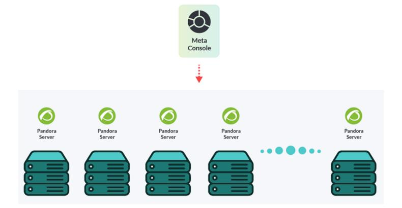
It is a complex environment, which incorporates the necessary functions to manage the different instances. The Command Center (Metaconsole) is designed not to manage at a low level, like the instances, but to operate with all the infrastructure that you have, centralizing all its nodes.
