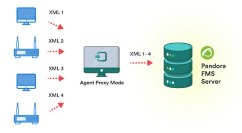
• Need to monitor different networks for remote monitoring with the server: In this case you can also use the Satellite Server or several different Pandora FMS servers connected to the same database.
