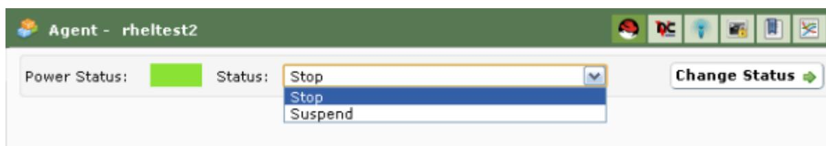
If you choose the Stop state to stop the virtual machine, the extension will connect to the RHEV API and send the command. The result will be the change of state in the virtual machine and the combo options.
