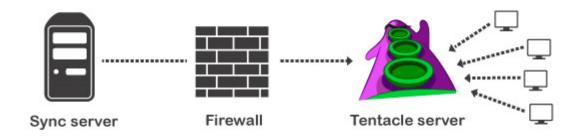
Start from Pandora FMS central server as if it were a standard installation. In the remote network, a data collection point (Tentacle server) is installed, which stores all data until the main server (Sync server) initiates communications and downloads the information, similar to a buffer.
